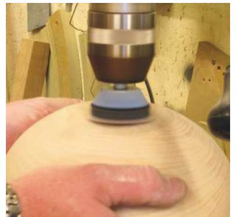
▲ Pic.18 With the remaining timber removed you will need to sand the bottom of the bowl. The best way is to mount your sanding arbor in the drill press, maintain a strong hold and keep it moving
